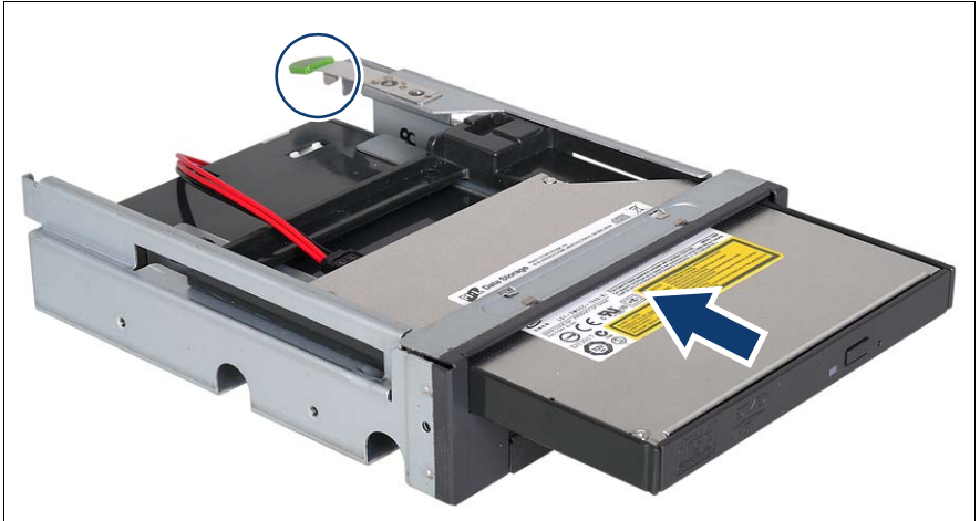
Figure 35: Inserting the DVD drive module in the Multibay 1
